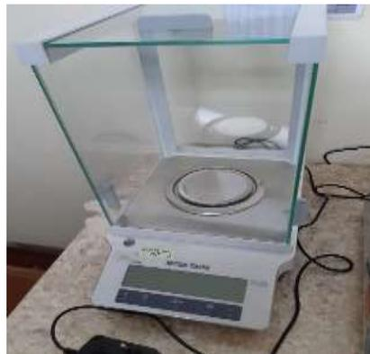
**Gambar 1. Timbangan Elektronik Mettler Toledo Kapasitas 6.200 gram**
